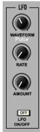
The LFO controls the **FREQUENCY(Cutoff)** of the Filter. LFO can be turned On and Off using the **LFO ON/OFF** button.
