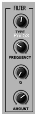
The **Filter** section has a Filter **TYPE** knob (with different Low Pass and High Pass filters), with **FREQUENCY(Cutoff)** and **Q (Resonance)** controls.
